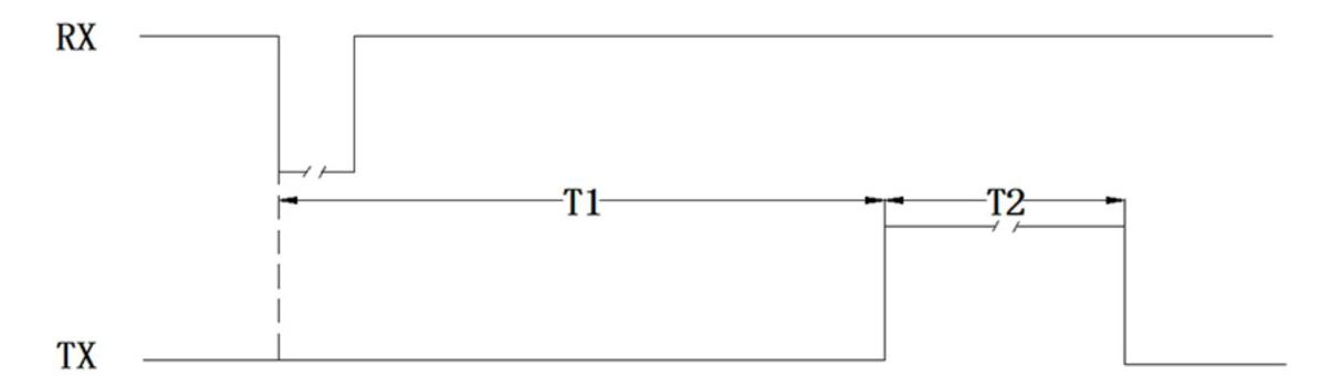
Remark: T1=0.9s~2.5s T2=1.4ms~80ms (Timing of PWM High-level pulse width ).Suggest timing between 10us and 2ms of RX falling edge pulse width.
