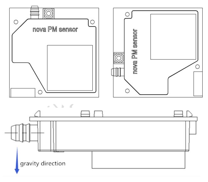
4. Hose connection: optional. It can be connected with the hose of 6mm inner diameter and 8mm external diameter. The hose cannot be longer
