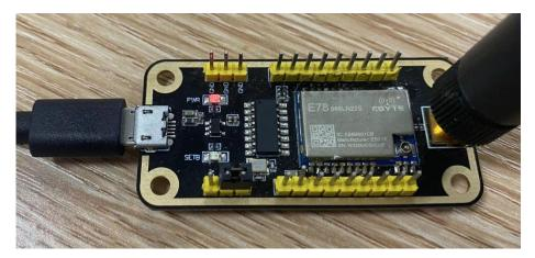
As shown in the figure, plug in the jumper cap and select 3.3V power supply. Both E78-915TBL-02 are configured in this way. Open the corresponding serial port to send and receive data.
