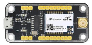
E78-915TBL-02 is a complete set of test products specially for E78 series SMD SOC modules combined with USB to TTL serial port backplane. All E78-868LN22S (6601) module pins have been drawn out for customer testing and development, which greatly reduces customer testing and development difficulty.
