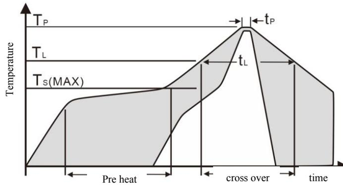
Figure 9. JEDEC standard soldering process diagram,  $T_P < 200^\circ\text{C}$ ,  $t_P < 30\text{sec}$ , lead-free soldering.  $T_L < 180^\circ\text{C}$ ,  $t_L < 150\text{sec}$ , and the rate of temperature rise and fall during soldering should be  $< 5^\circ\text{C}/\text{sec}$ .
