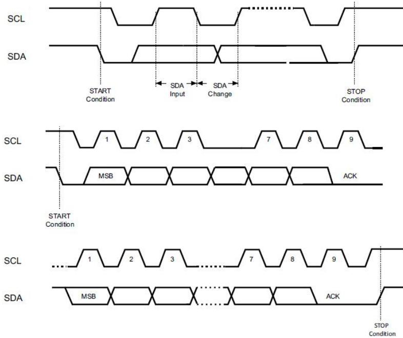
Figure 17. I<sup>2</sup>C bus timing diagram
