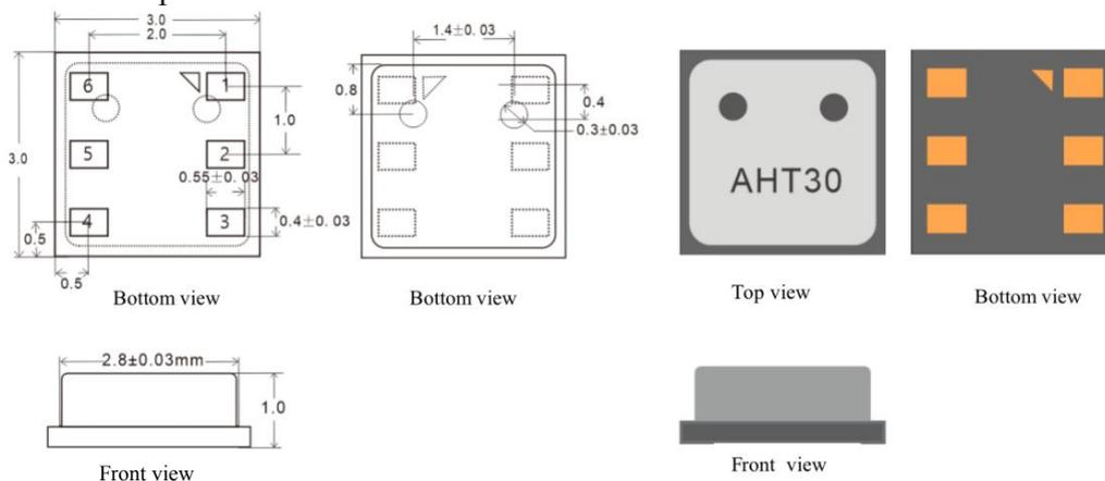
Figure 1: AHT30 temperature and humidity sensor (Unit: mm Tolerance: ±0.1 mm)
