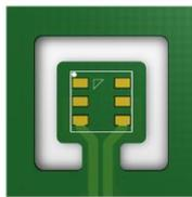
Figure 10. Top view of the sensor PCB with milled slits to minimize heat transfer.
