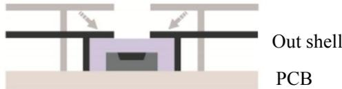
Figure 13. The smaller measurement blind zone the better, which is beneficial for the sensor to quickly and comprehensively detect environmental changes.
