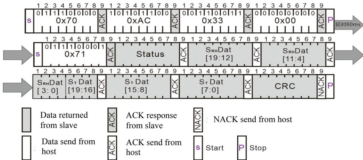
0x70 0xAC 0x33 0x00 is to send the write measurement command byte segment to the sensor;
