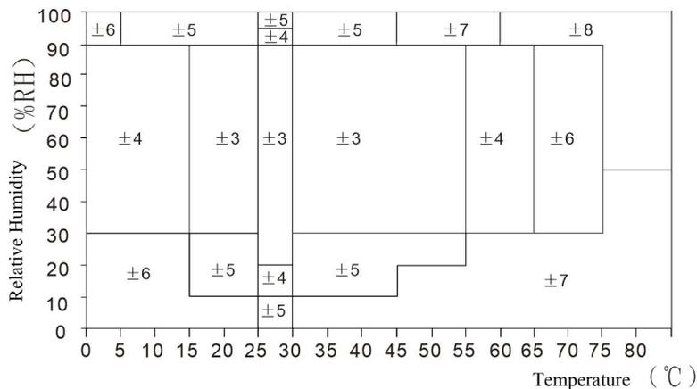
Figure 5. Typical error of relative humidity in the range of 0~80°C Δ%RH
