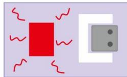
Figure 14. Isolating the sensor from internal heat sources minimizes the effect of internal heat on sensor measurements.
