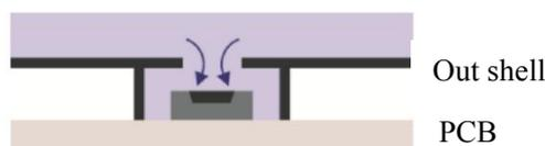
Figure 11. A suitable window on the housing provides good access for ambient measurements and more air exchange.
