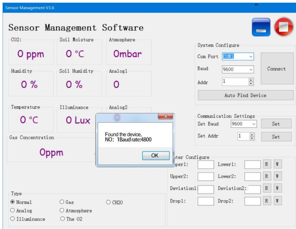
Please note that this software can only test one device at the same time. After connecting the physical device, click the **CONNECT** button to read the information. In the UNCONNECT state, you can modify BAUD and ADDR in COMMUNICATION SETTINGS.
