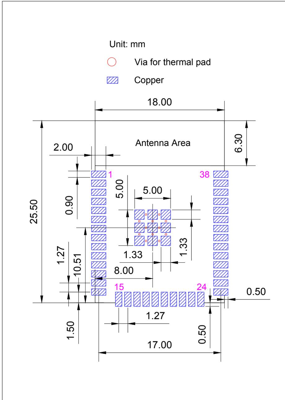
Figure 8: Recommended PCB Land Pattern of ESP32-SOLO-1
