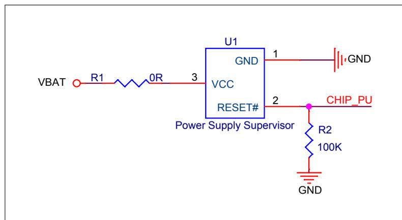
Figure 6: Reset Circuit
