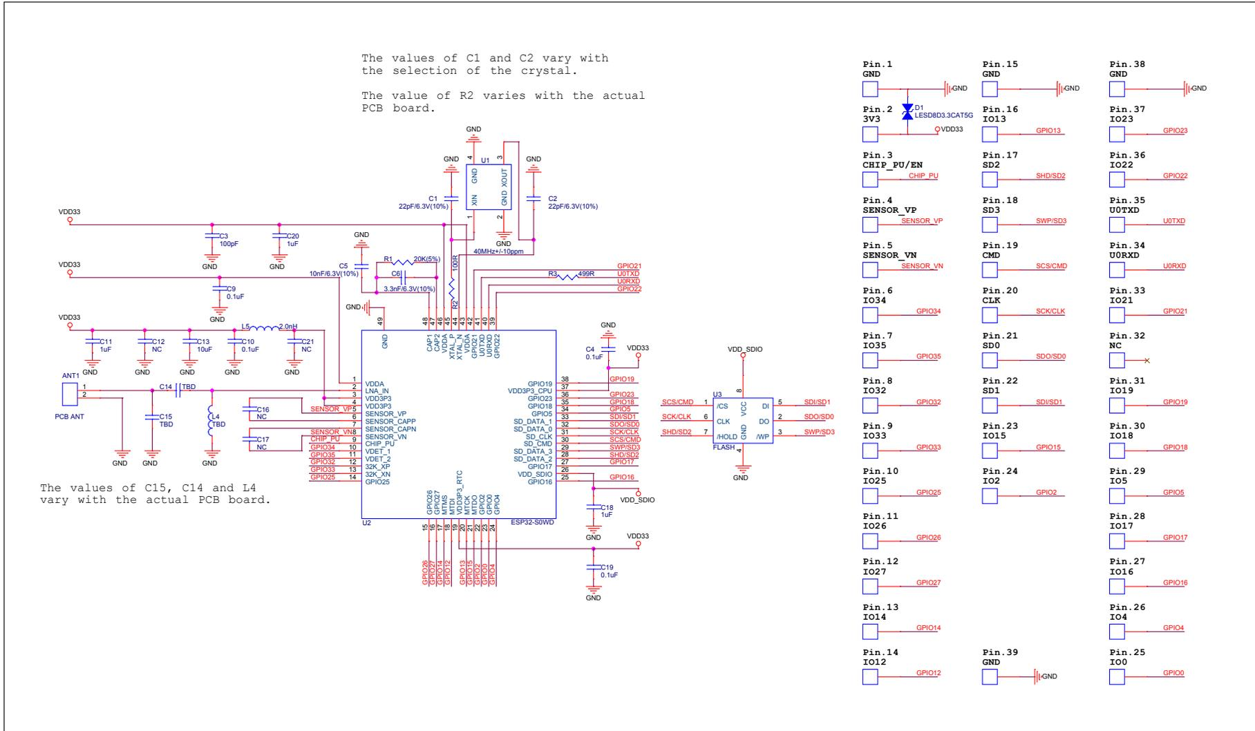
Figure 3: ESP32-SOLO-1 Schematics
