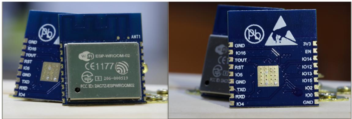
Figure 1-1. ESP-WROOM-02 Module
