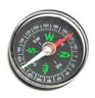
The compass is placed on the horizontal table, and after the compass is still, the red pointer points to the North Pole. Slowly rotate the outer casing so that the bottom North Pole and arrow overlap.
