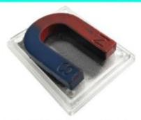
Place the different magnets on the iron powder box, tap the iron powder box gently, and observe the shape of the iron powder in the iron powder box.
