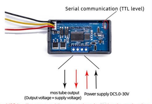
Note: MOS is a live output, and the output voltage is equal to the supply voltage.
