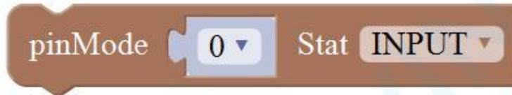
Set the IO pins as Output or Input state
