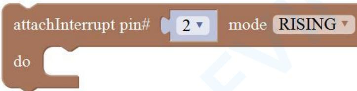
External Interrupts function, with three trigger interrupt modes RISING, FALLING, CHANGE.
