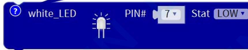
Connect the LED light module to the digital port D7, control the D7 port to output low level, turn off the light
