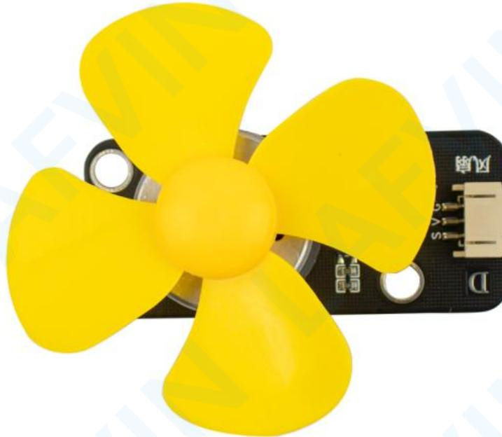
The motor fan module has three pin interfaces, G means GND grounding, V means VCC Connect to high level, S is the control signal input pin, which can be connected to the Arduino control board. Word port. The fan speed can also be adjusted by connecting the PWM signal pins of the digital port (D3 D5 D6 D9 D10 D11).
