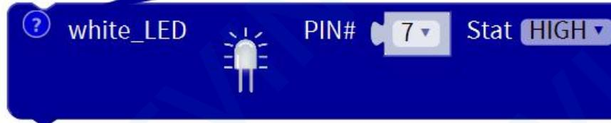
Connect the LED light module to the digital port D7, control the D7 port to output high level, turn on the light
