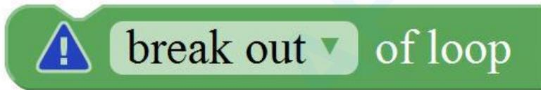
break function, used to exit from the containing loop.
