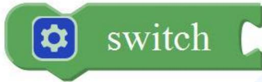
**switch** function. You can click the blue gear icon to select the **case** block or **default** block. (used to evaluate several programs then execute the corresponding function matched with program.)
