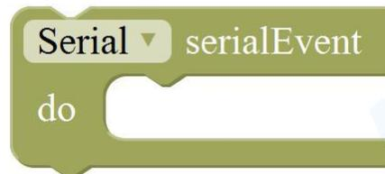
Event function trigger by serial port data, that is, serial port is ready to call this function. (equal to an interrupt function)
