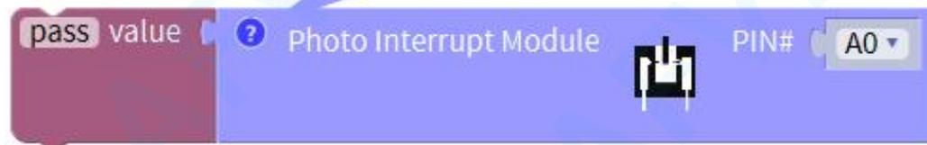
Photoelectric interrupt Module is connected to the analog port A0. When a coin is inserted, the program block outputs a low level "0", when no coin is inserted, the program block outputs a high level "1", and the obtained value is saved to the variable pass.
