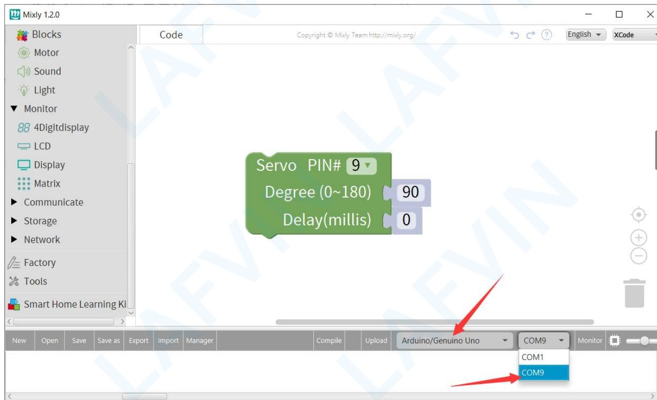
After completing the program upload, connect the servo motor to the digital interface D9, and the servo motor will execute the command to rotate to the 90 degree position. (This is also the default position of the servo motor when it leaves the factory)
