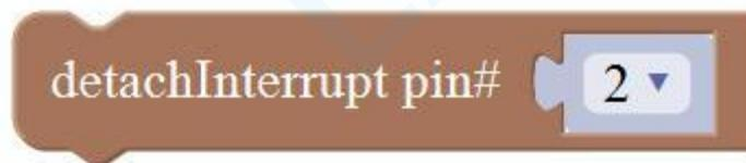
Detaches interrupt to a specific Port. Turn off the given interrupt function.
