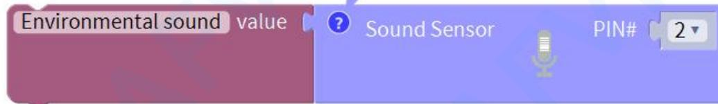
The sound sensor module is connected to the digital port D2 and compares the received sound intensity with the set threshold. When it is greater than the threshold, the program block directly outputs a high level "1"; when it is less than the threshold, the program block directly outputs the bottom voltage Level "0" and save the obtained level state to the variable Environmental sound
