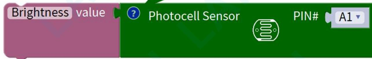
The photosensitive sensor is connected to the analog port A1. The photosensitive sensor converts the light intensity into an analog voltage value (0~1024), and the program block directly outputs a value in the range of 0~1024. Save the obtained value to the variable Brightness.
