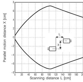
● 1.5mm dia. slit mounted at receiver
