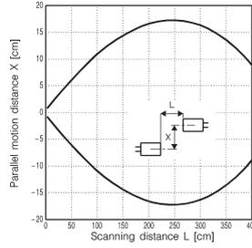
● 3mm dia. slit mounted at both emitter and receiver
