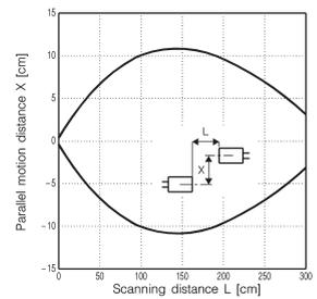
● 1mm wide horizontal slit mounted at both emitter and receiver
