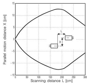
● 1mm wide vertical slit mounted at receiver
