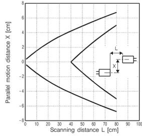
● 3mm dia. slit mounted at emitter
