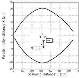
● 1.5mm dia. slit mounted at emitter
