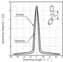
● Scanning distance characteristics (typical values) when slit HPJ-U01 is attached (comparison with slit not attached)
