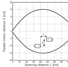
● 2mm wide horizontal slit mounted at both emitter and receiver
