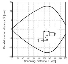
● 1.5mm dia. slit mounted at both emitter and receiver
