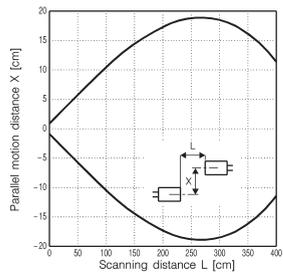
● 2mm wide vertical slit mounted at both emitter and receiver
